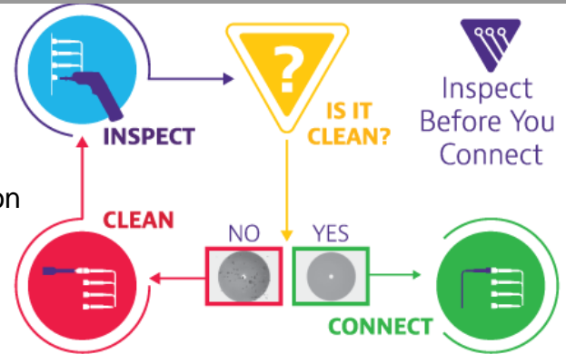
Figure 13: Inspect Before You Connect
